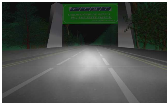
Figure 5: Headlights simulation over the highway created with the real texture of asphalt.
