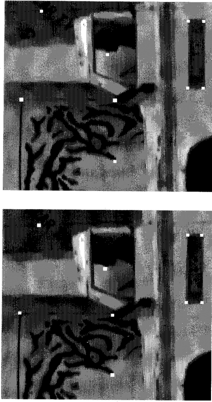
Figure 7.1 An illustration of the correspondence problem. A matching between corresponding points of an image pair is established (only some correspondences are shown).
