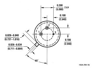
TO-39 Metal Can Package (H) Order Number LM78M05CH, LM78M12CH or LM78M15CH NS Package Number H03A
