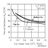
FIGURE 3.  $\theta_{\text{JA}}$  vs. 2oz Copper Area for TO-252
