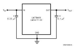
\*Required if regulator input is more than 4 inches from input filter capacitor (or if no input filter capacitor is used).
