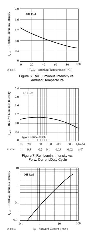
Figure 8. Relative Luminous Intensity vs. Forward Current
