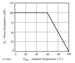
Figure 1. Power Dissipation vs. Ambient Temperature
