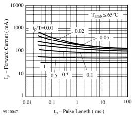
Figure 3. Forward Current vs. Pulse Length
