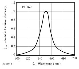
Figure 9. Relative Luminous Intensity vs. Wavelength
