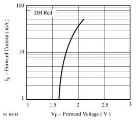
Figure 5. Forward Current vs. Forward Voltage
