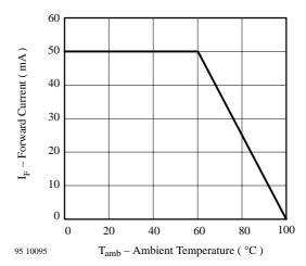
Figure 2. Forward Current vs. Ambient Temperature
