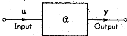
Fig. 1.2.1 Diagrammatic representation of a system G with input u and output y .
