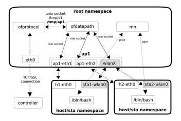
Fig. 1. Components and connections in a two-host network created with Mininet-WiFi.
