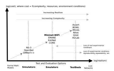
Fig. 6. Overview of related work and trade-offs of different wireless experimental platforms.
