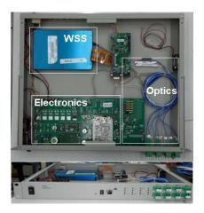
Fig. 3. Testbed WSS ROADMs line card
