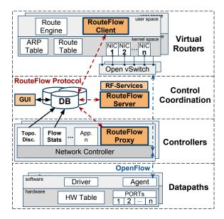
Figure 2: Architecture design of the RFCP.
