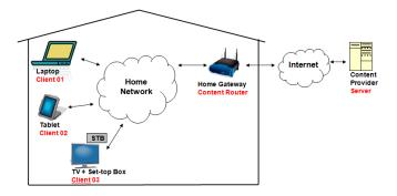
Fig. 6. Home Network Experiments. Three clients requesting content over a wireless link with a single CR acting as the Wifi access point and home gateway to the Internet.
