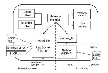
Fig. 1. CR Internal Modules
