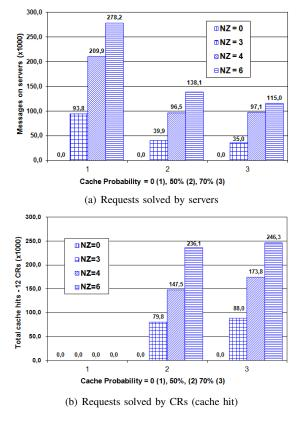
Fig. 3. REQUEST messages handling (Ethernet)
