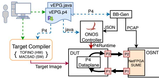
Figure 5: Testbed for vEPG evaluation on HW and SW.
