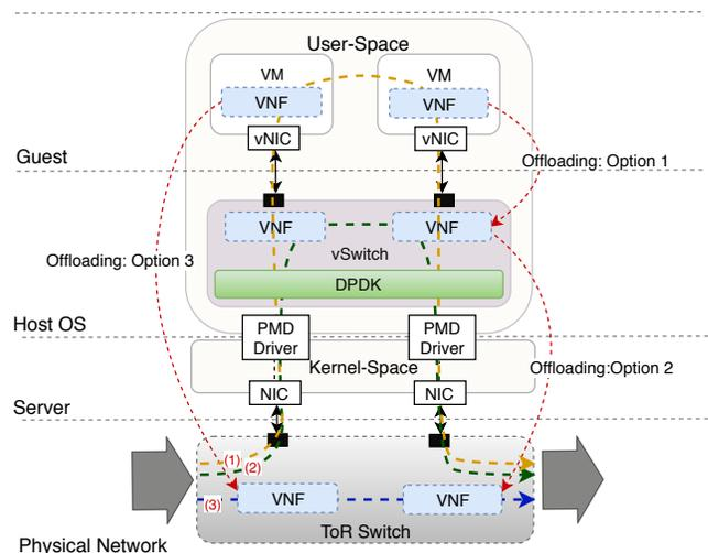
Figure 1: Performance bottlenecks in NFV infrastructure and VNF offloading options in multi-tenant environment to accelerate packet-processing functions
