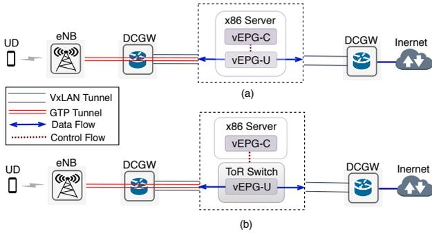
Figure 3: vEPG offloading use case : vEPG-U running on (a) x86 server and (b) Barefoot Tofino ToR switch.
