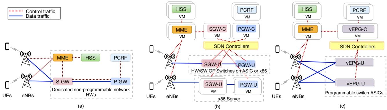
**Figure 2: MPC architecture implementation alternatives: (a) Traditional MPC appliances, (b) MPC using SDN and NFV with full and partial virtualization, and (c) MPC user plane functions offloaded to programmable ASICs.**
