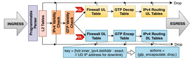
Figure 4: P4-defined vEPG pipelines featuring the main Up-link (UL) and Downlink (DL) tables
