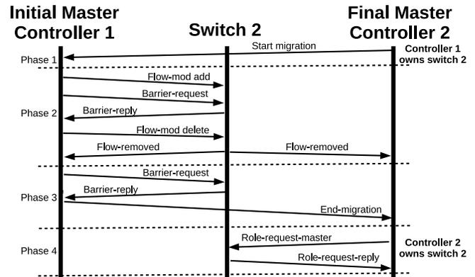
Fig. 2. Protocol Failure Repair.
