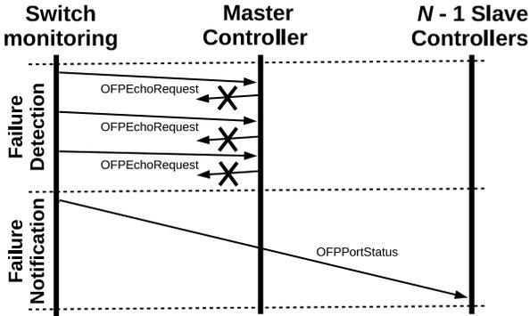
Fig. 3. Failure Detection from switches.
