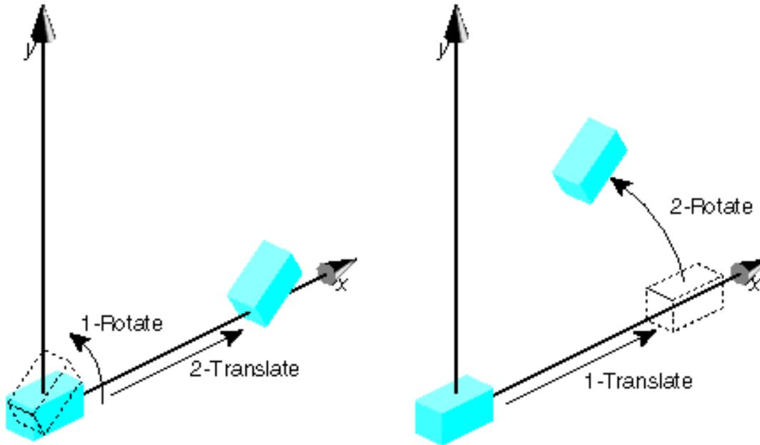
$$P' = T.(R.P) = (T.R).P \quad P' = R.(T.P) = (R.T).P$$
