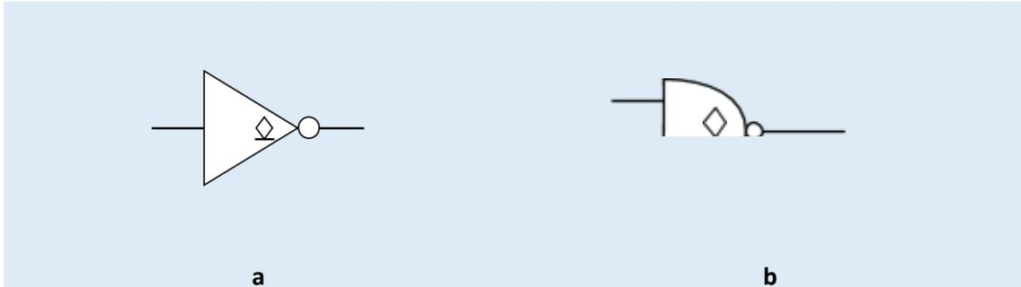
Figura 2.14 - Símbolos de gates com Open Collector/drain (a) Inversor (b) NAND
