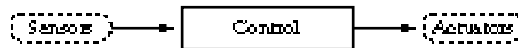
Figure 3.2.1 A behavior module is defined as a transformation from sensory input and to actuator output.
