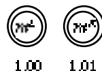
Figure 3.4.3 The ‘network’ that generates the basic move behavior. Only the two output nodes are needed. Since the resting activity of the left node (1.00) is slightly lower than that of the right (1.01), the creature will move in a large circle.
