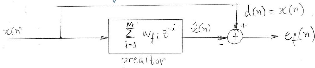
$$\hat{x}(n) = w_{f_1} x(n-1) + w_{f_2} x(n-2) + \dots + w_{f_M} x(n-M) = w_f^T \underline{x}(n-1)$$
