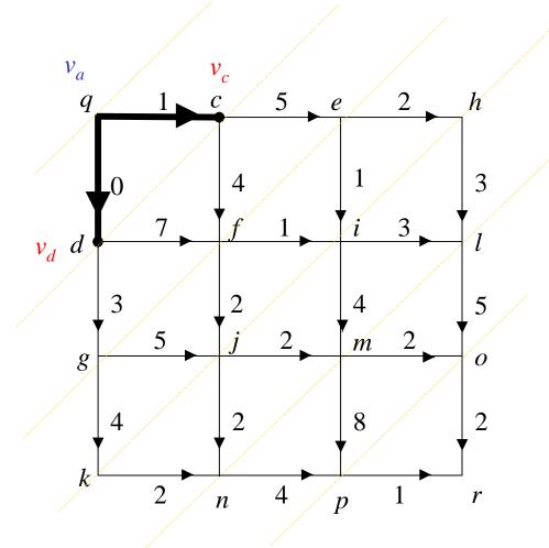
$$v_{q} = \min \{1 + v_{c}, 0 + v_{d}\}$$
