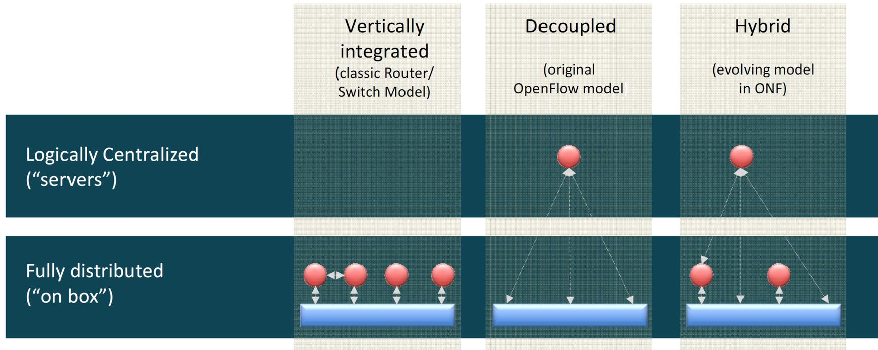
Data Path jointly controlled by standard on-box control plane and centralized off-box controller
