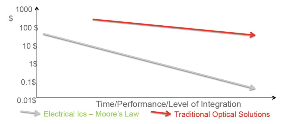
Optics ~25 years behind Electronics – level of integration, manufacturability etc & Gap is widening due to orders of magnitude larger investment in infra-structure
