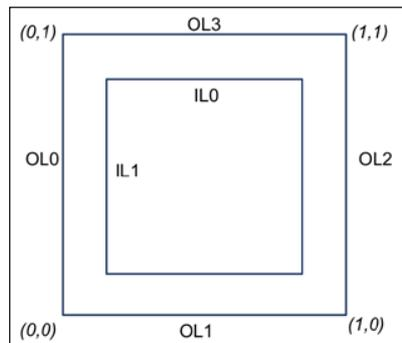
The six tessellation levels described some time back can be configured via the arrays `gl_TessLevelOuter` and `gl_TessLevelInner`. For example, `gl_TessLevelInner[0]` corresponds to **IL0**, `gl_TessLevelOuter[2]` corresponds to **OL2**, and so on.
