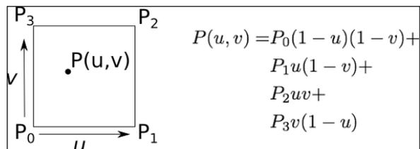
We'll let the tessellation primitive generator create a set of vertices with appropriate parametric coordinates, and we'll determine the corresponding positions by interpolating the corners of the quad using the preceding equation.
