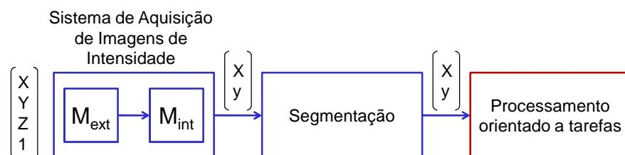
$$M_{int} M_{ext} = \begin{pmatrix} -f/s_x & 0 & o_x \\ 0 & -f/s_y & o_y \\ 0 & 0 & 1 \end{pmatrix} \begin{pmatrix} r_{00} & r_{01} & r_{02} & t_x \\ r_{10} & r_{11} & r_{12} & t_y \\ r_{20} & r_{21} & r_{22} & t_z \end{pmatrix}$$
