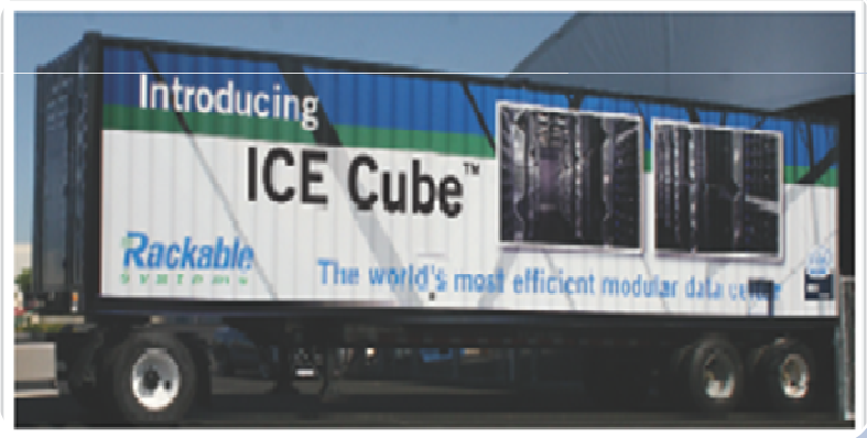
Rackable Systems Container 2800 servers in 40'
