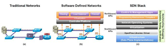
Figure 1. (a) Traditional networks with distributed control and device-specific management contrast with (b) the flexible and logically-centralized control and management in SDN enabled networks due to southbound protocols (e.g. OpenFlow, RESTCONF, PCE-P, etc...) that interact with data plane devices, enabled by (c) an emerging SDN stack based on open APIs between functional layers in addition to a number of supporting tools.
