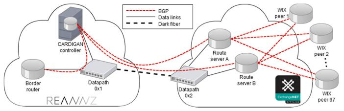
Figure 3. The logical router interconnection between REANZ and WIX is implemented with the Cardigan controller (running a tailored version of RouteFlow) to control two OpenFlow switches (Datapath 0x1 and 0x2) physically interconnected through dark fiber.
