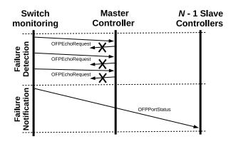
Fig. 3. Failure Detection from switches.
