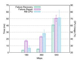
Fig. 5. Impact of the load at dataplane for recovery and repair.
