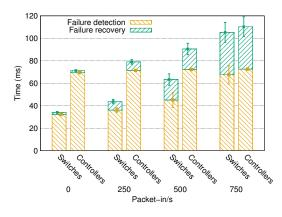
Fig. 6. Failure detection and recovery from controllers vs. from switches.
