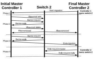
Fig. 2. Protocol Failure Repair.
