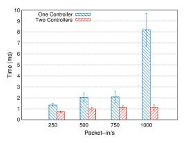
Fig. 7. Latency for packet-in processing with one and two controllers. D. Emulated Environment: Latency versus Replication
