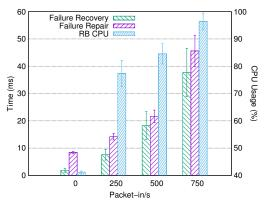
Fig. 4. Time to failure recovery and repair varying packet-in/s.
